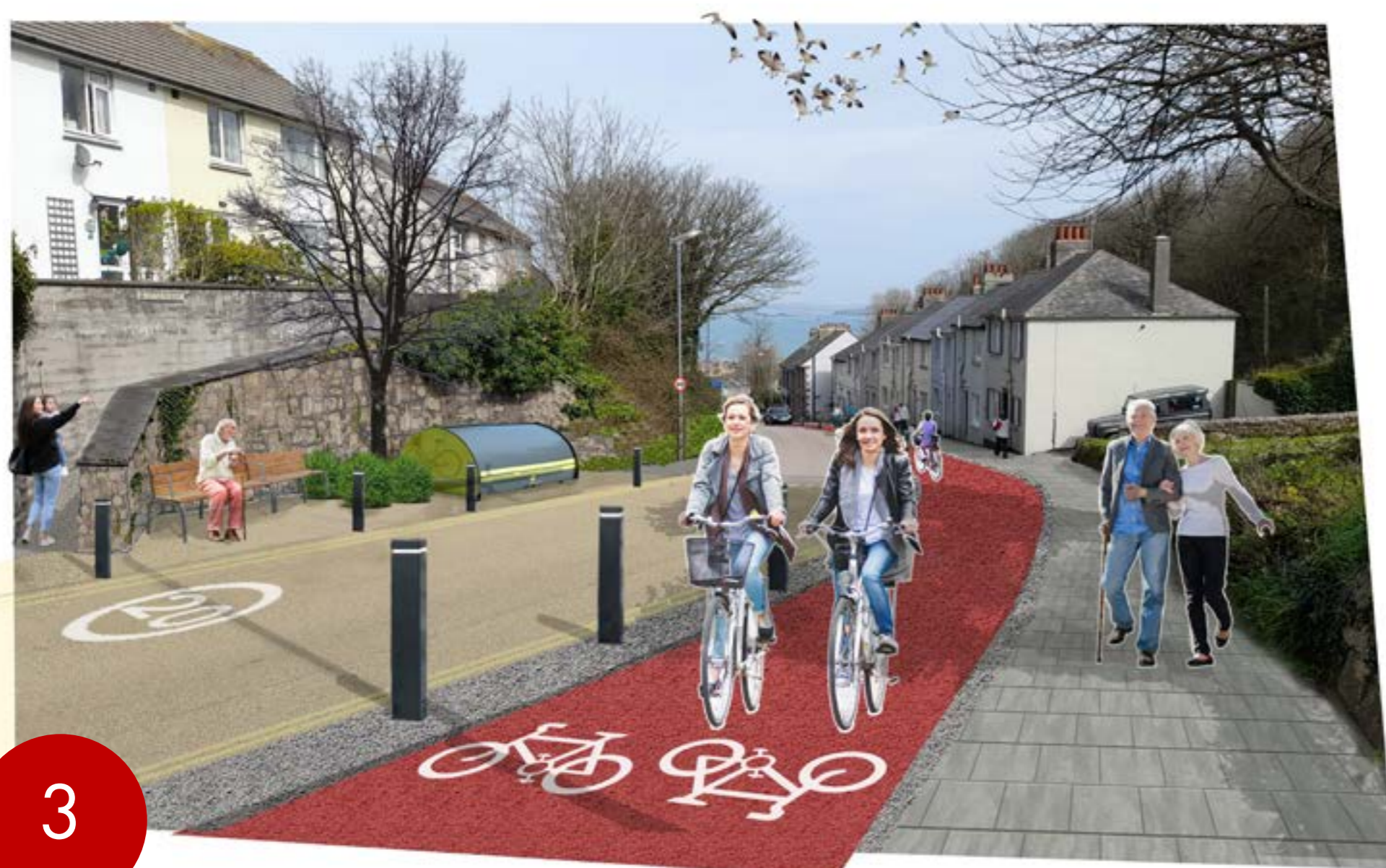
High Stennack - 2 way cycle track and narrowed carriageway to slow vehicles and make walking easier.
