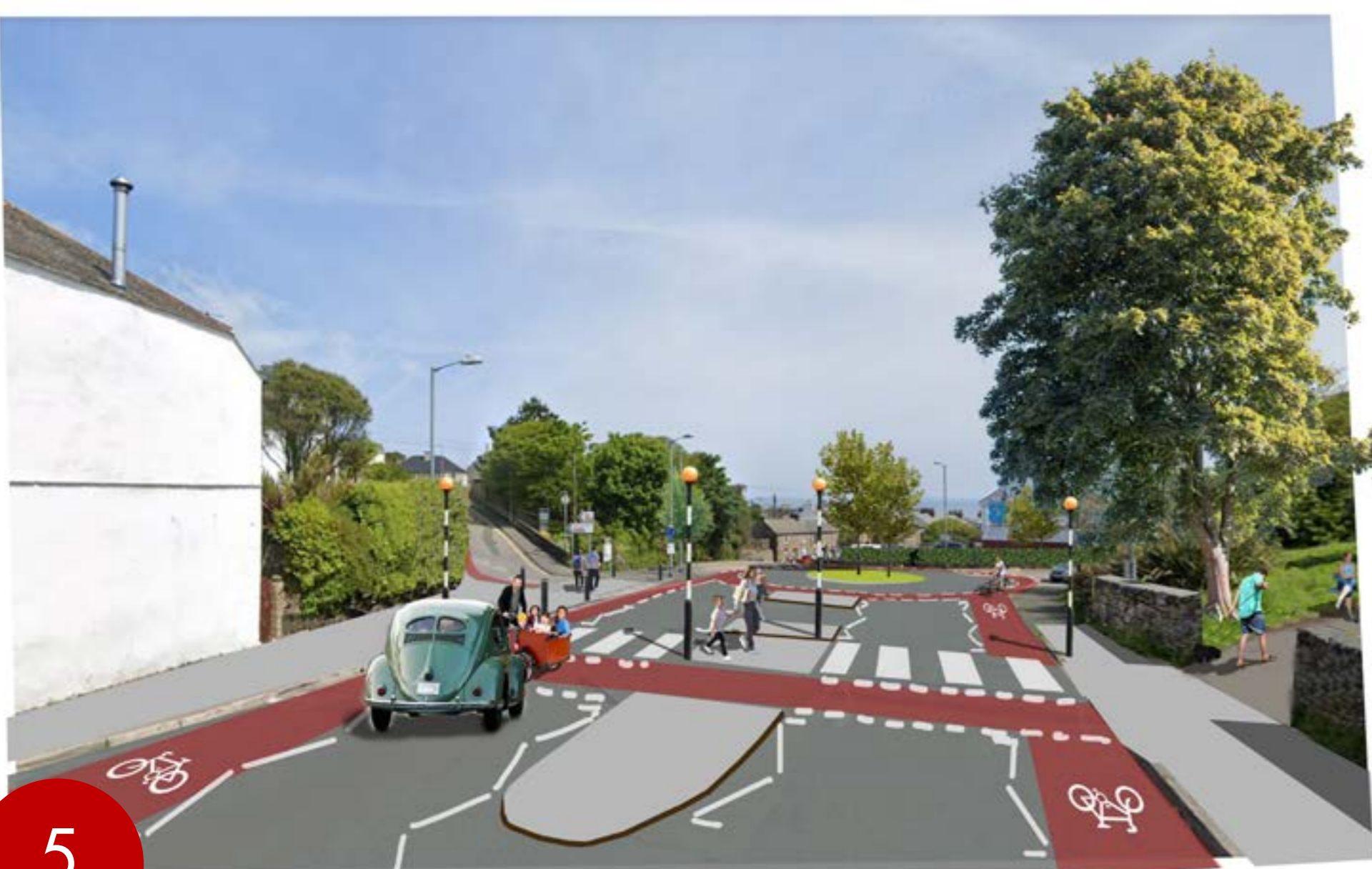
Higher Stennack/ Carnellis Road at the upper town Co-op - parallel cycle crossing and cycle roundabout
