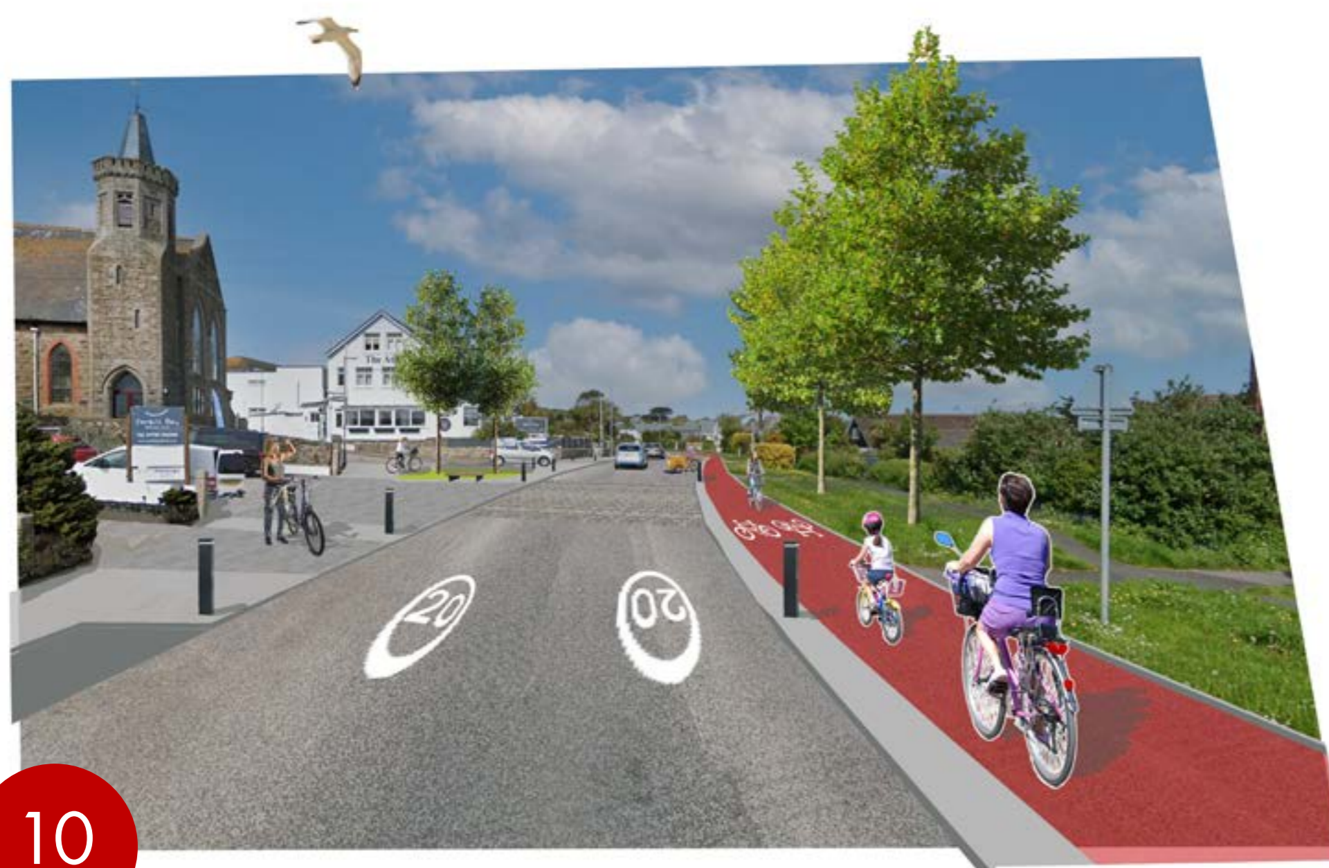
St Ives Road, Carbis Bay - 2 way cycle track and wide junction bellmouths reduced in size to create more pedestrian space. Tree planting would give summer shade and help provide shelter from winds.
